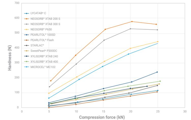
Figure 3: Filler-binder excipient compactability, as measured using Korsch® XP1 with 13mm diameter concave punches at 20 tablet/min rate.
