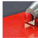
Cross cuts + tape peeling
