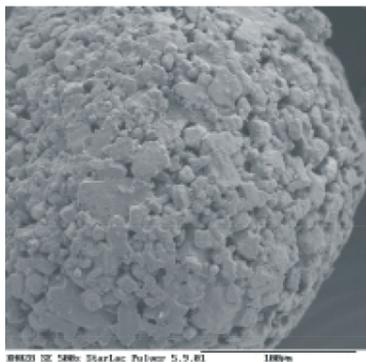
The mean particle size of StarLac® (Fig. 6) and FlowLac®, both the D50-data and the distribution of particle size, differ scarcely. Maize starch consists of smaller particles in comparison to the other materials. The densities and the resulting parameters describe, that the good flowability of StarLac® is similar to that of FlowLac®. Both Hausner ratio and Carr-Index increase in the order FlowLac® < StarLac® << maize starch.
