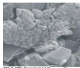
Figure 5. SEM of tablets of StarLac® at 0.95 maximum relative density at 15000 magnification.
