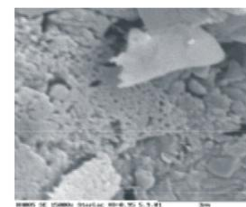
The SEMs show the difference before (Fig.4) and after (Fig.5) tableting of StarLac®. The powder of StarLac® has regular crystals of lactose (A), embedding crystals of lactose in the amorphous lactose (B) and a starch particle (C). After deformation the crystals are smaller and the particle of starch create a fine net work. A reason of this phenomenon can be the viscoelastic flow of starch at high pressure, because only at a maximum relative density of 0.95 this can be detected.
